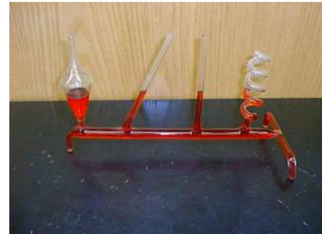
$$P = \frac{F}{A} = \frac{m * g}{A} = \frac{\varphi * V * g}{A} = \frac{\varphi * A * h * g}{A} = \varphi * g * h$$
