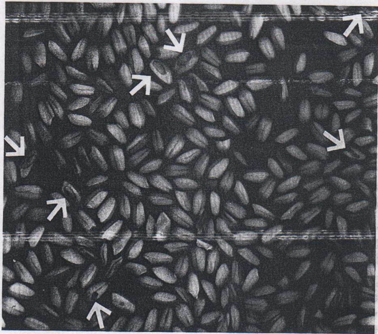
Fig. 12. X-ray of wheat, showing internal infestation (arrows).
