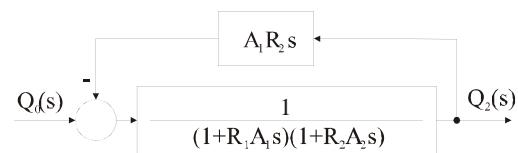
$$Q_0(s) \rightarrow \frac{1}{1+s(R_1A_1+R_2A_2+R_3A_3)+s^2(R_1R_2A_1A_2)} \rightarrow Q_2(s)$$
