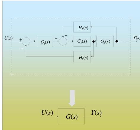
$$G(s) = \frac{G_1(s)G_2(s)G_3(s)}{1 + G_2(s)G_3(s)H_2(s) + G_1(s)G_2(s)H_1(s)}$$
