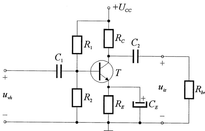
$$\begin{aligned} R_1 &= 39 \text{ k}\Omega \\ R_2 &= 12 \text{ k}\Omega \\ R_C &= 2,2 \text{ k}\Omega \\ R_E &= 560 \Omega \\ R_{br} &= 1,5 \text{ k}\Omega \\ h_{11e} &= 2 \text{ k}\Omega \\ h_{21e} &= 120 \\ h_{12e} &= 10^{-3} \\ h_{22e} &= 10^{-4} \text{ S} \\ C &= \infty \\ C_E &= \infty \end{aligned}$$
