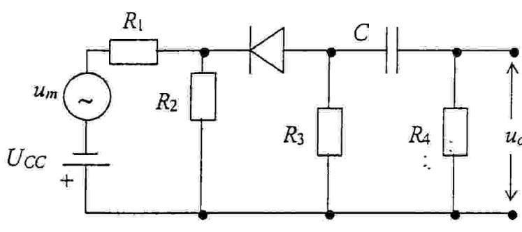
$$\begin{aligned}R_1 &= 8 \Omega \\R_2 &= 32 \Omega \\R_3 &= 24 \Omega \\R_4 &= 180 \Omega \\C &= 100 \mu F \\U_{CC} &= 1,5 V \\u_m &= U_m \cos \omega t \\U_m &= 50 \text{ mV}; \omega = 10^4 \text{ rad/s} \\r_D &= \frac{U_T}{I_{DQ}}; U_T = 25 \text{ mV}\end{aligned}$$
