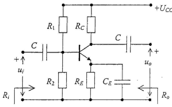
$$\begin{aligned}R_1 &= 20 \text{ k}\Omega \\R_2 &= 30 \text{ k}\Omega \\R_C &= 2,4 \text{ k}\Omega \\R_E &= 500 \Omega \\h_{11e} &= 1,2 \text{ k}\Omega \\h_{21e} &= 80 \\h_{12e} &= h_{22e} = 0 \\C &= \infty \\C_E &= \infty\end{aligned}$$
