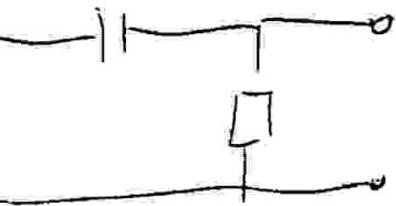
$$H(j\omega) = \frac{U_o(j\omega)}{U_i(j\omega)} = \frac{R}{R + \frac{1}{j\omega C}} = \frac{\omega^2 R^2 C^2 + j\omega RC}{1 + \omega^2 R^2 C^2}$$
