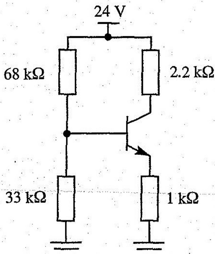
5.6 Determine the value of  $R_C$  to ensure that  $V_{CE} \geq 3$  V if  $\beta$  varies from 80 to 240. Assume that  $V_{BE} = 0.7$  V.
