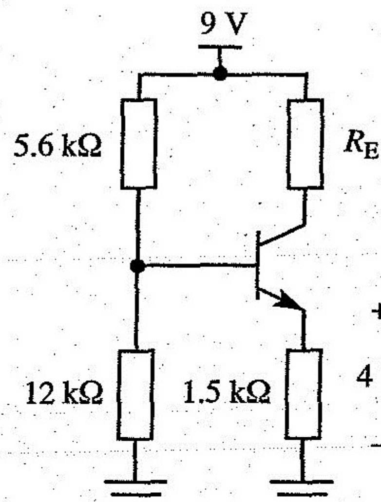
5.14 Determine the collector current for the pnp emitter-biased circuit if  $\beta = 120$  and  $V_{BE} = 0.7$  V.
