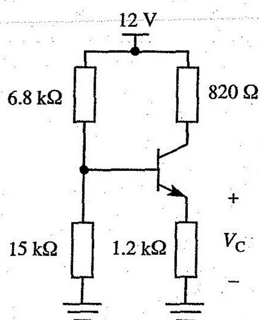
5.13 If  $V_{CE} = 5$  V,  $\beta = 250$  and  $V_{BE} = 0.7$  V, determine  $R_B$ .
