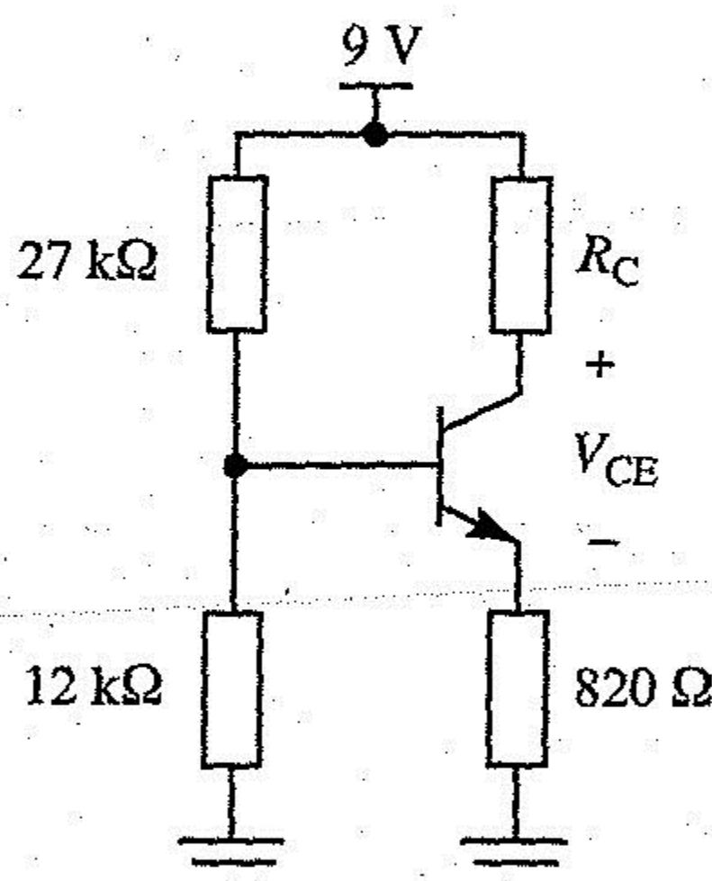
5.7 Determine the change in  $V_{CE}$  if  $\beta$  varies from 120 to 420. Assume that  $V_{BE} = 0.7$  V.
