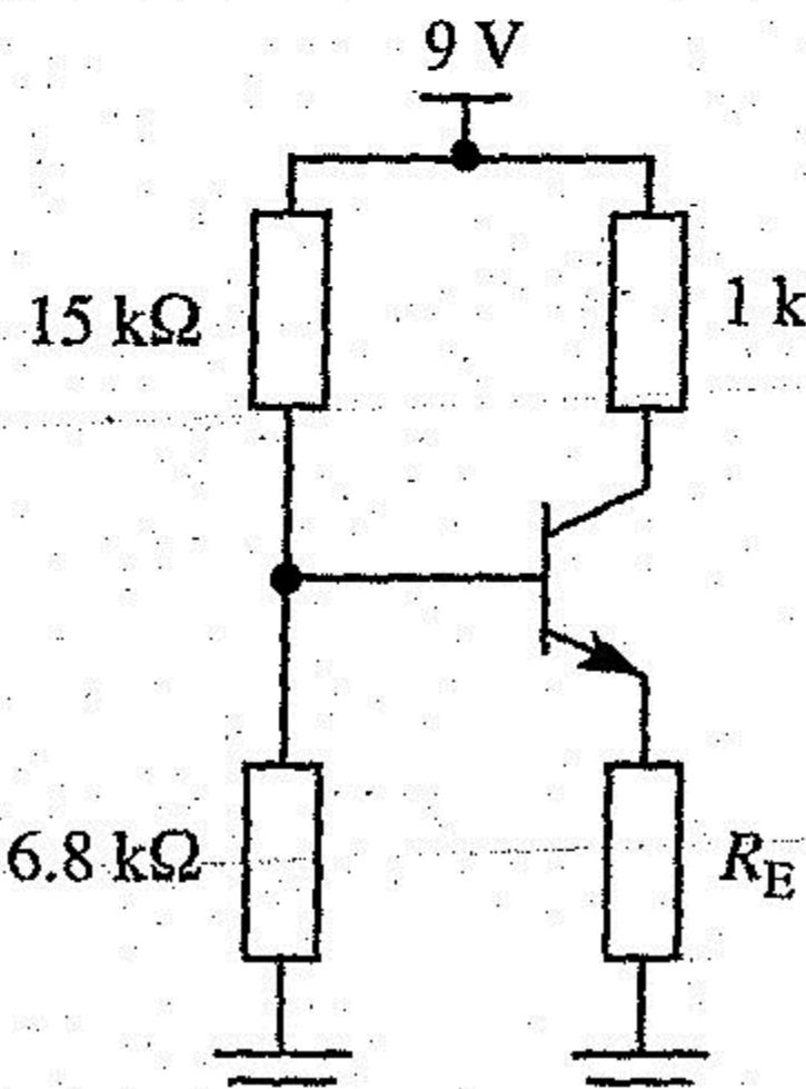
5.9 For the circuit shown  $\beta = 120$  and  $V_{BE} = 0.7$  V. Verify that the collector current is 1.1 mA and determine the value of  $R_E$  which is required to provide a collector current of 2 mA.
