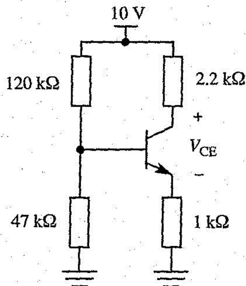
5.8 Select a suitable value for  $R_E$  to provide a collector current of 2 mA if  $\beta = 150$  and  $V_{BE} = 0.7$  V.
