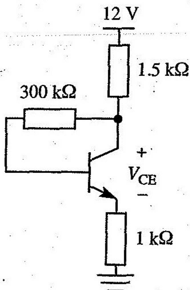
5.15 Determine  $V_C$  if  $\beta = 150$  and  $V_{BE} = 0.65$  V.
