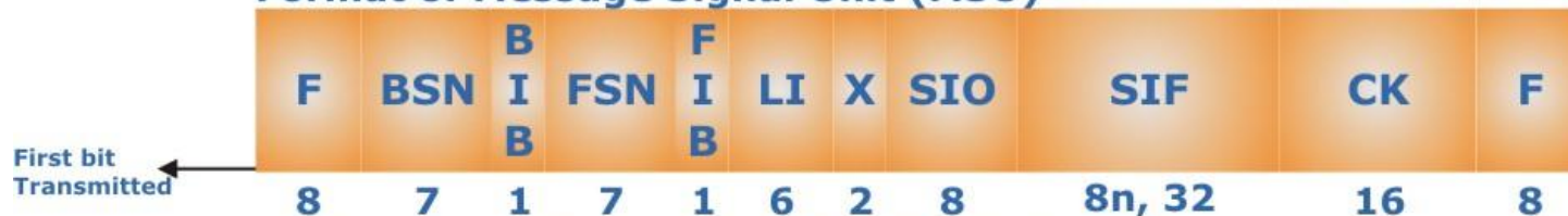
Format of Link Status Signal Unit (LSSU)
