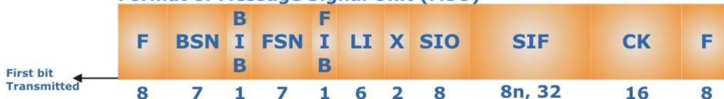
Format of Link Status Signal Unit (LSSU)
