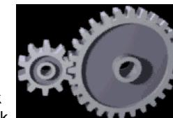
$$g_r = \frac{R}{r} = \frac{\Omega}{\omega} = \frac{\omega}{\Omega} = \frac{M_r}{P} = \frac{M_R}{M_r}$$
