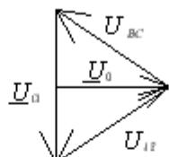
$$\underline{U}_0 = \frac{\underline{U}_{CA}}{2} + \underline{U}_{AB} = \frac{\sqrt{3}}{2} 400 \text{ V}$$
