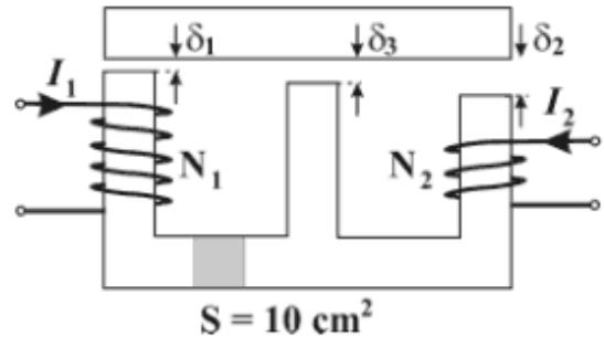
$$\Phi_3 = \Phi_2 - \Phi_1; \quad R_{\delta 1} = \frac{\delta_1}{\mu_0 S}; \quad R_{\delta 3} = 2R_{\delta 1}; \quad R_{\delta 2} = 3R_{\delta 1}$$
