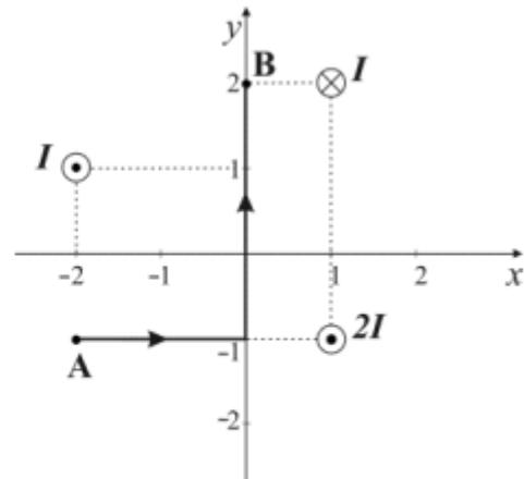
$$\Theta_{AB} = \int_A^B \vec{H} d\vec{l} = \frac{I}{2\pi} \left( \frac{\pi}{2} + \arctg \frac{1}{2} \right) + \frac{I}{2\pi} \frac{\pi}{4} - \frac{2I}{2\pi} \arctg 3 = 0,05 \text{ A}$$
