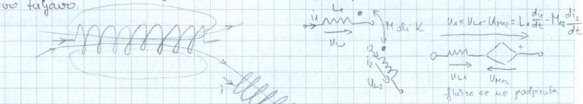
$$\begin{aligned} M_{12} &= k \sqrt{L_1 L_2} \\ U_{M12} &= -U_{M21} \\ U_1 &= U_{L1} - U_{M12} = L_1 \frac{di_1}{dt} - M_{12} \frac{di_2}{dt} \\ U_2 &= U_{L2} + U_{M21} = L_2 \frac{di_2}{dt} + M_{12} \frac{di_1}{dt} \end{aligned}$$
