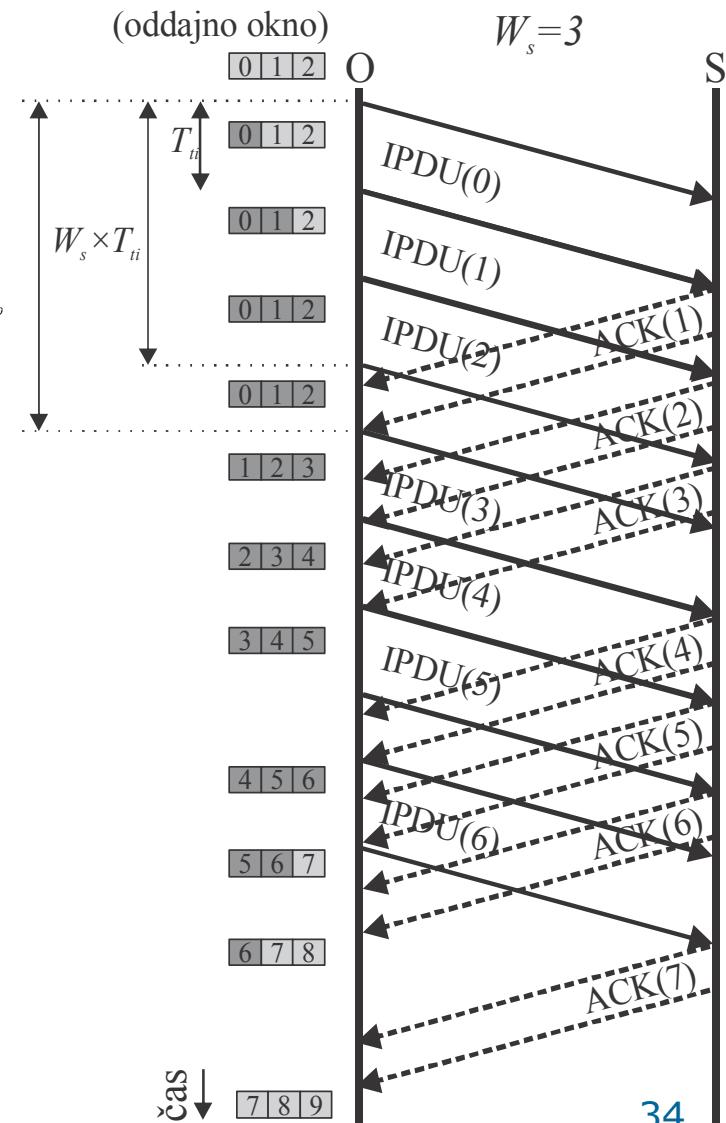
$$\eta = \frac{W_s \cdot T_{ti}}{T_{rt}} = \frac{W_s \cdot T_{ti}}{T_{ti} + T_{ta} + 2 \cdot T_p}$$
