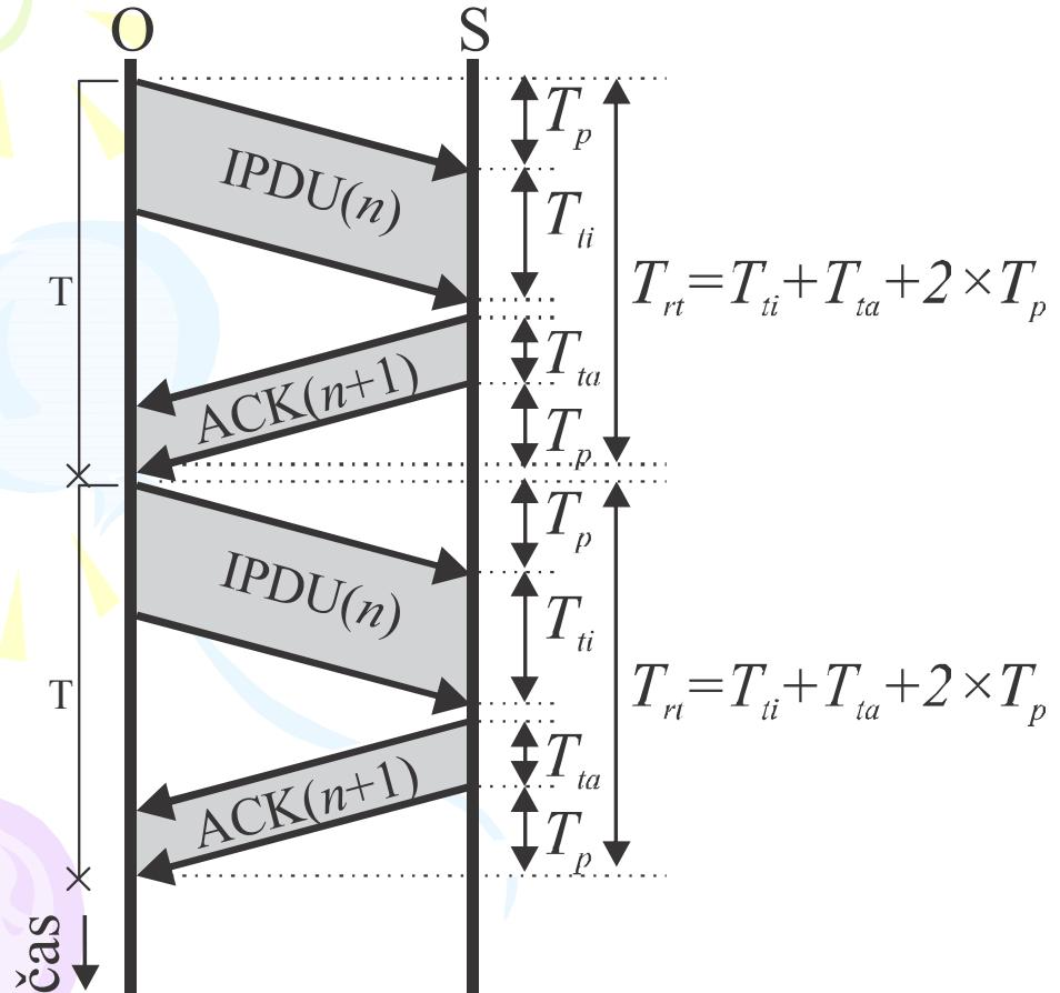
$$\eta = \frac{t_{ti}}{t_{rt}} = \frac{t_{ti}}{t_{ti} + t_{ta} + 2 \cdot t_p}$$
