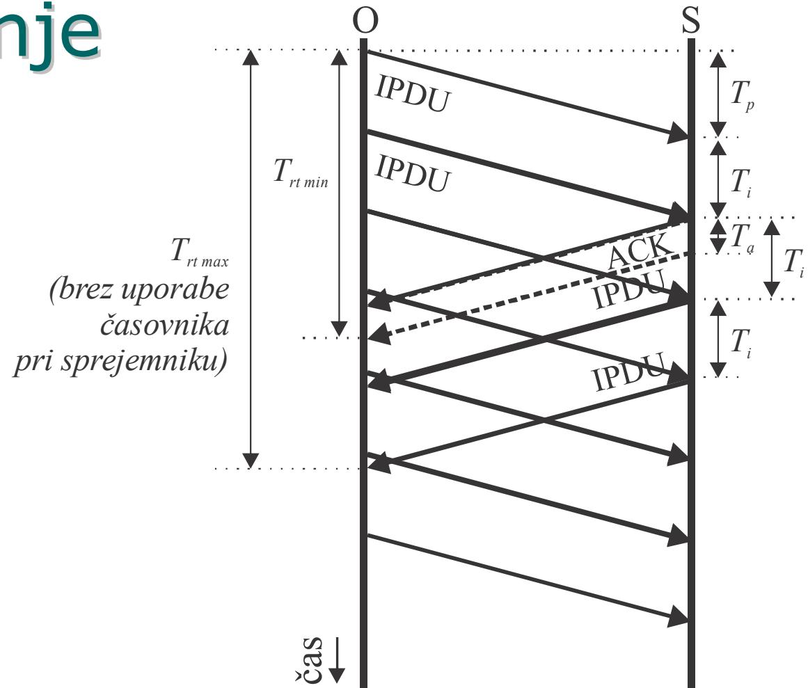
$$t_i + t_a + 2 \cdot t_p \leq t_{rt} \leq 2 \cdot t_i + 2 \cdot t_p + t_{tor}, \quad t_{tor} \geq t_i$$
