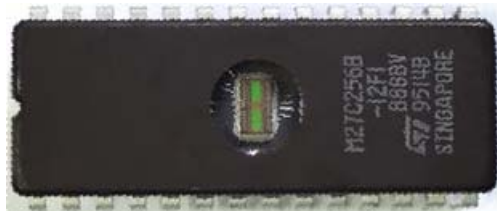
32 KB (256 Kbit) EPROM M27C256B (ST Microelectronics)
