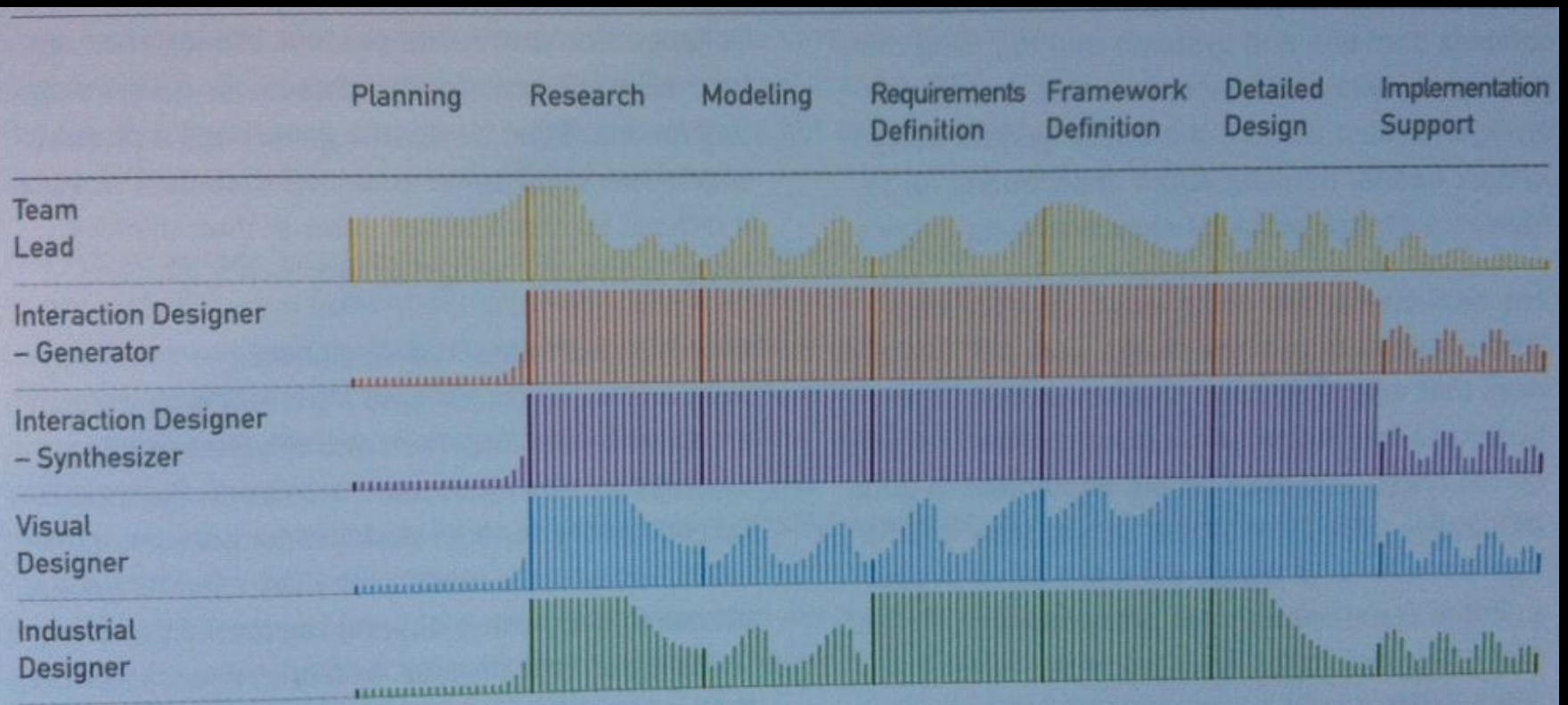
Figure 2.2. An overview of design team member involvement. The team lead may be the only designer involved in project planning. Thereafter, the two interaction designer roles are full-time, and the industrial designer and visual designer are involved at least part-time in every activity, more if budget allows. The team lead maintains some involvement throughout.
