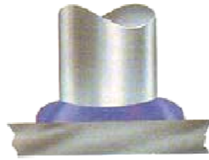
4. Metal solidifies and weld is completed in milliseconds.
