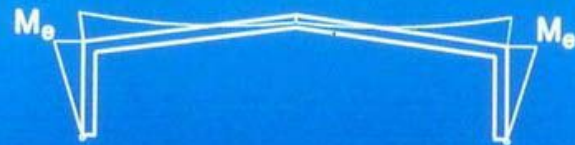
Elastic analysis of prismatic frame (Pre 1950)
