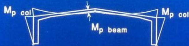
Plastic analysis of haunched frame (Post 1960)
