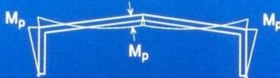
Plastic analysis of prismatic frame (1950-60)
