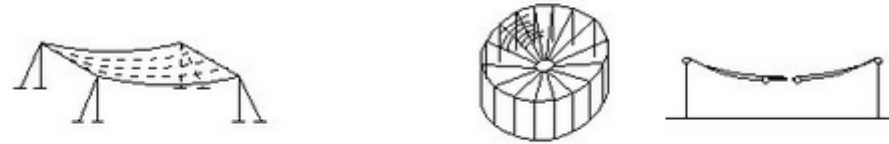
Parallel cable system
