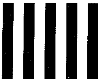
Fig. 4.3. Typical object used to determine the resolution of a photographic system in terms of line-pairs per unit length.
