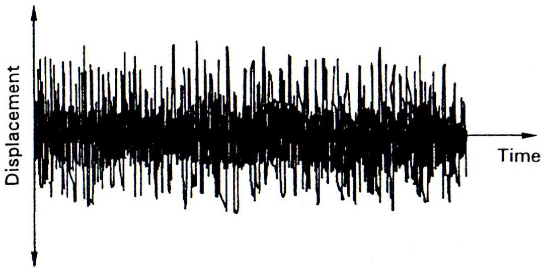
FIGURE 7.4.3 Noise waveshape
