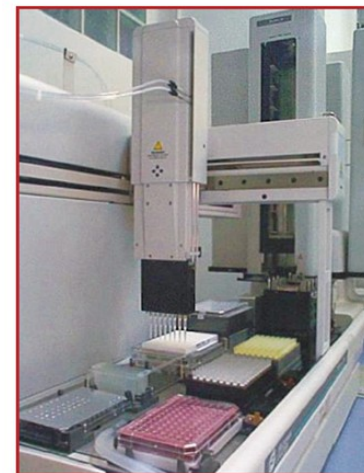
Figure 1B. Automated SELEX process using a standard Biomek 2000 workstation.
