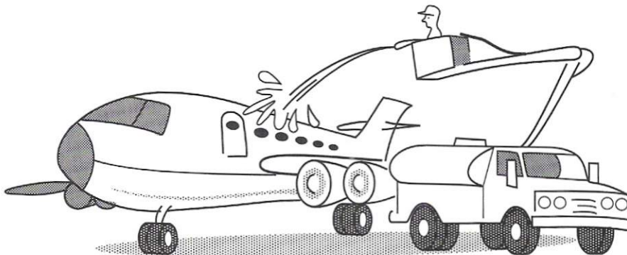
Figure 2.1-2. Deicing Aircraft. Snow is removed by spraying the planes with a 70°C aqueous solution of 50 wt. % ethylene glycol. We seek an alternative deicer that can be recycled.
