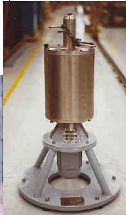
2. Podbielniak centrifugal extractor POD. (Courtesy of Baker Perkins, Inc., Michigan [38])
