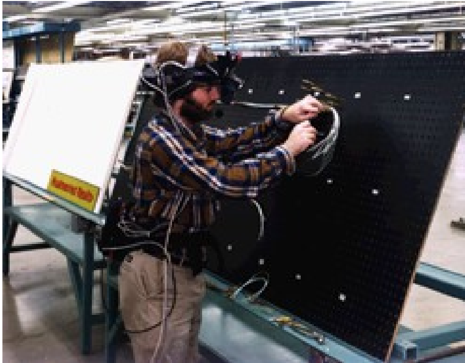
Boeing wire harness assembly. Adam Janin wearing HMD. Courtesy David Mizell, Boeing
