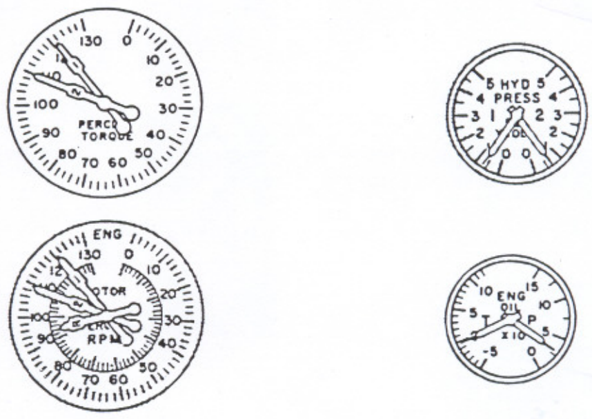
Figure 1.7 Dual-indicator displays. The display with three pointers has a helicopter application: it shows the speed of No. 1 and No. 2 engines, and of the main rotor.
