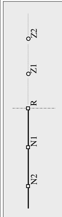
$$\begin{aligned} \frac{dw}{dx}(x_R) &\approx D^1 w_R = \frac{w_{Z1} - w_{N1}}{2h} \\ \frac{d^2w}{dx^2}(x_R) &\approx D^2 w_R = \frac{w_{Z1} - 2w_R + w_{N1}}{h^2} \\ \frac{d^3w}{dx^3}(x_R) &\approx D^3 w_R = \frac{w_{Z2} - 2w_{Z1} + 2w_{N1} - w_{N2}}{2h^3} \end{aligned}$$
