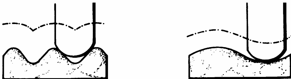
A rounded skid does not provide a serviceable datum if the surface irregularities are too widely spaced.
