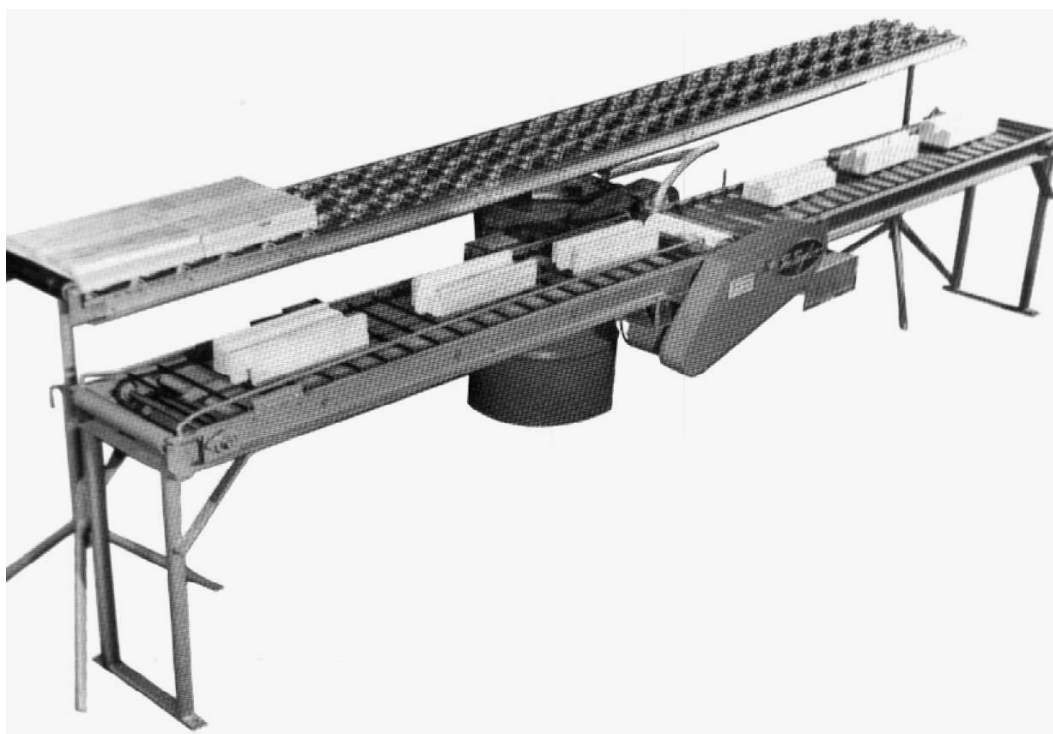
5.4.03 Slika: strojno nanašanje lepila; (James L.,TAYLOR , Manufacturing Company, Poughkeepsie, NY 12602-0712 USA )
