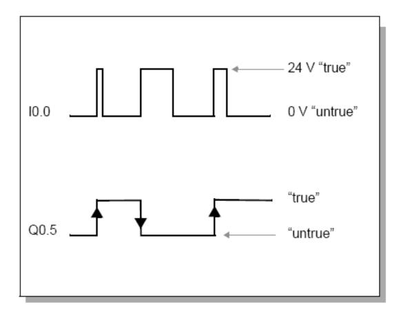
Detect whether a change of state from "0" to "1" (= positive edge) has taken place at I0.0.
