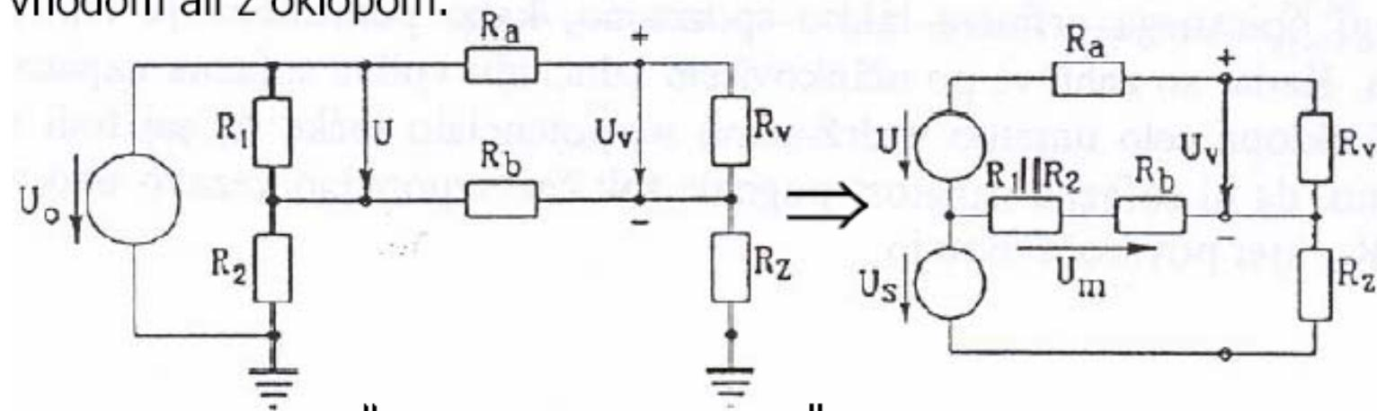
$$U_m = U_s \frac{R_1 \parallel R_2 + R_b}{R_1 \parallel R_2 + R_b + R_z} \approx U_s \frac{R_1 \parallel R_2 + R_b}{R_z}$$
